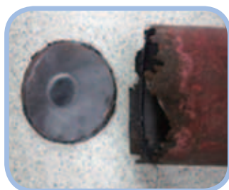
Corrosion existing in the shell
